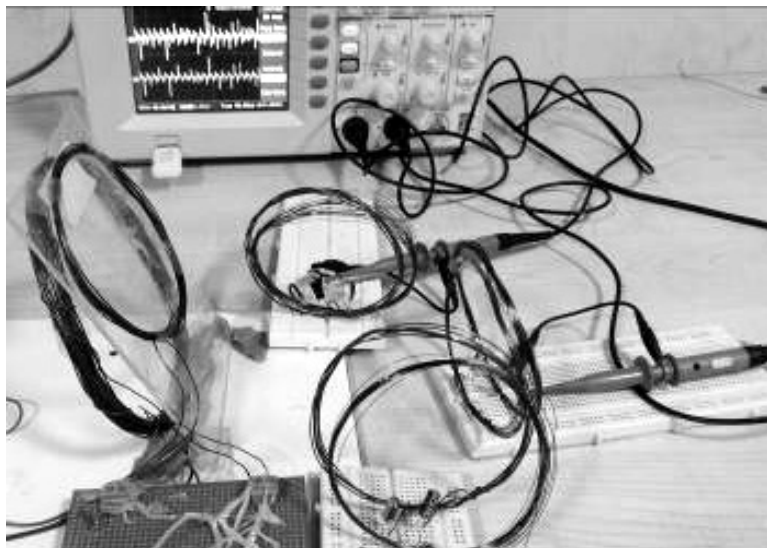
Figure 4: Experimental Setup of 3 Rx in at different angle with Tx
