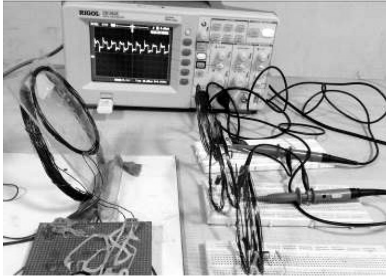
Figure 3: Experimental Setup of 3 Rx in Parallel with Tx
