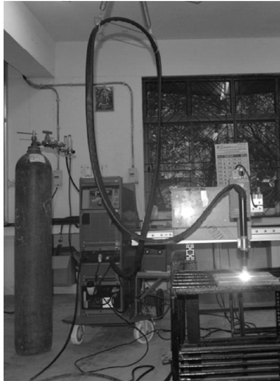
Figure 1: Image showing GTA Welding Experimental Setup
