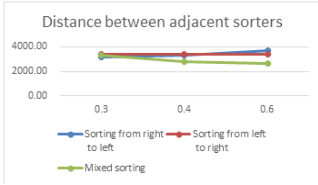
Fig.7 Comparison of the influence of distance (m) between adjacent sorters on the total sorting time of three sorting methods
