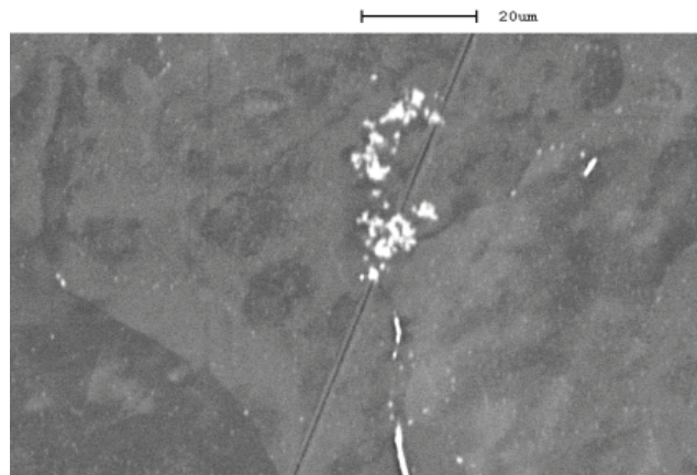
Figure 17. Scandium reinforced (0.4wt %) aluminium alloy with PMF (180 volt).
