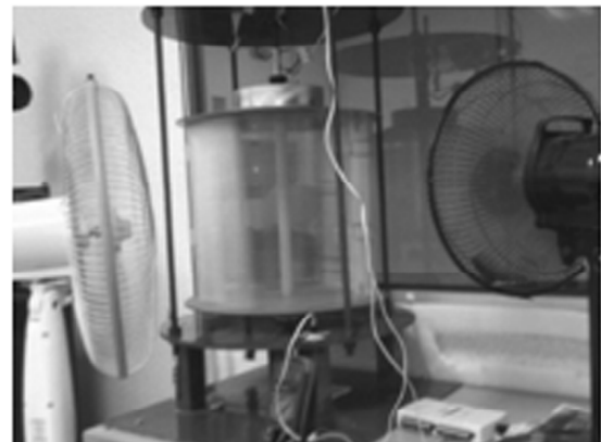
Figure 1: Hardware Architecture-Design of VAWT and PMSG
