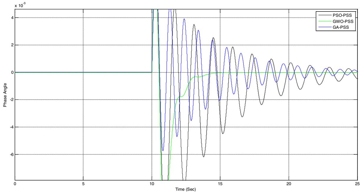
Figure 15: Comparison of Phase Angle Deviations in SMIB for GA-PSS, PSO-PSS and GWO-PSS
