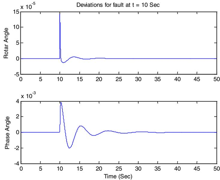
**Figure 18: Rotorangle Andphase Angle Deviation Of Hybrid Model (PSS-FOPID)**
