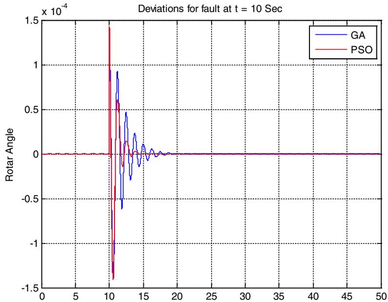
Figure 20: Comparison of Rotor Angle Deviations in SMIB for GA and PSO
