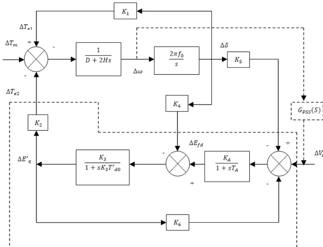
Figure 3: Heffron-Philips model of a system (Single-Machine Infinite-Bus System)
