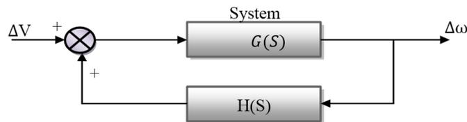
Figure 4: The Closed-Loop System (PSS)
