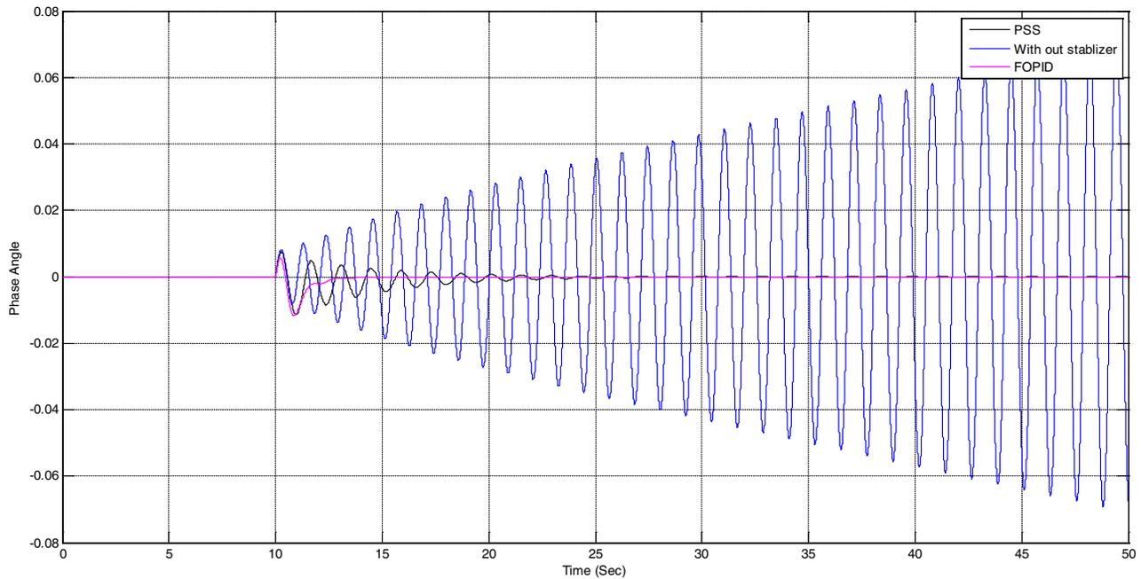
Figure 13: Comparison of Phase Angle Deviations in SMIB for PSS and FOPID
