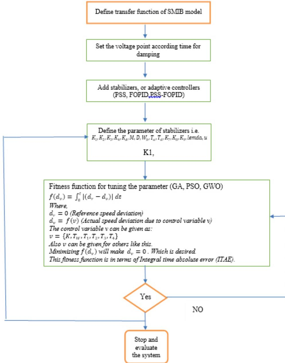
Figure 7: Flow of the Parameter Optimization of SMIB System Model
