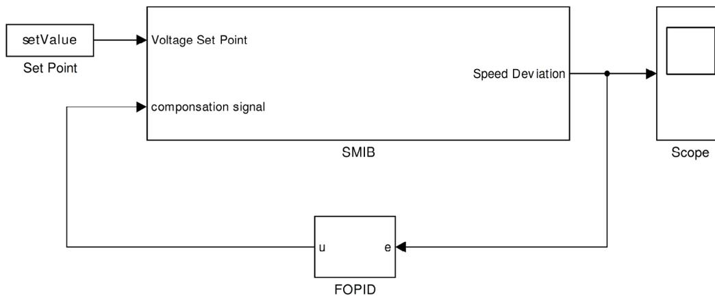
Figure 6: Simulink Model for SMIB with FOPID
