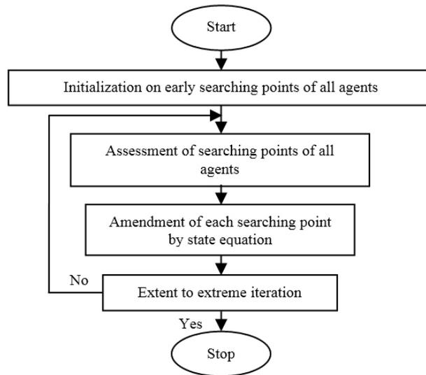
Figure 9: Flow Chart of PSO Algorithm
