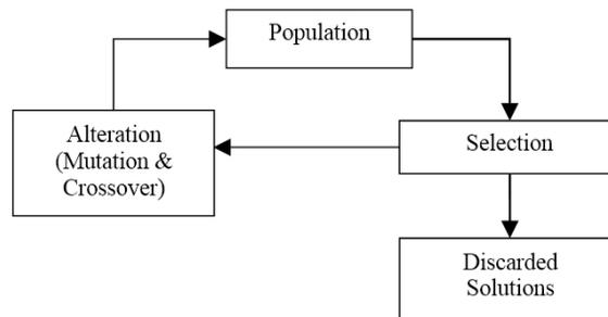
Figure 8: Genetic Algorithm Evolutionary Cycle
