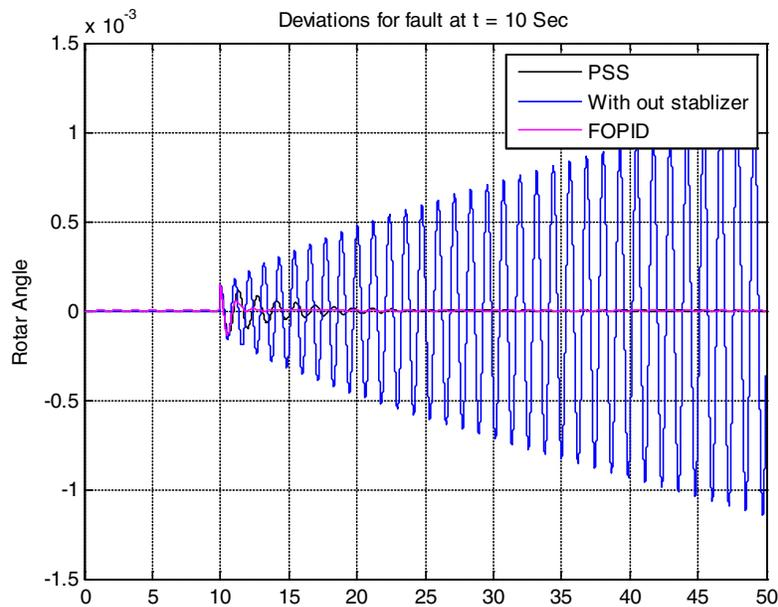
Figure 14: Comparison of Rotor Angle Deviations in SMIB for PSS and FOPID
