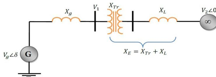
Figure 2: Synchronous Generator Connected to a Bus [24]
