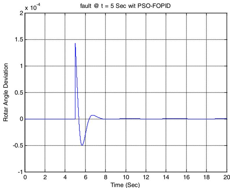
Figure 17: Rotor Angle Deviation for PSO-FOPID
