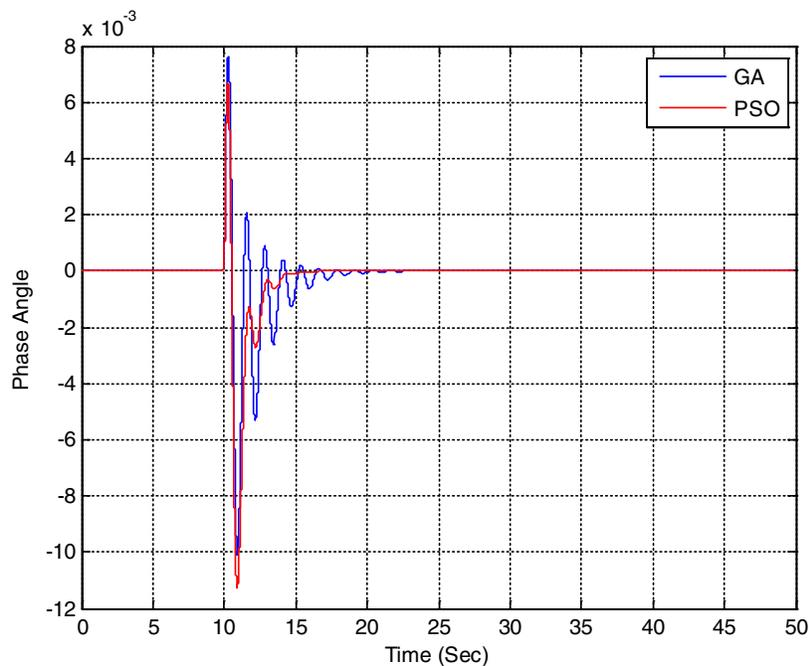
**Figure 19: Comparison of Phase Angle Deviations in SMIB for GA and PSO**
