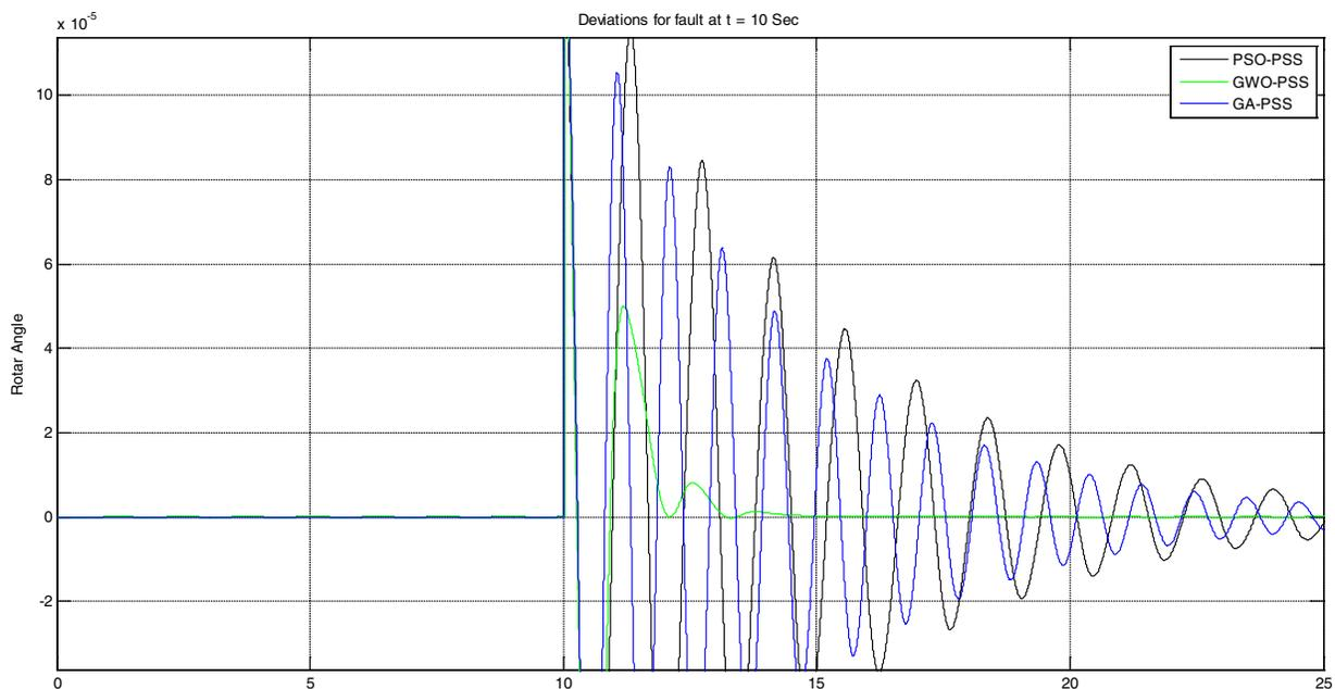
Figure 16: Comparison of Rotor Angle Deviations in SMIB for GA-PSS, PSO-PSS and GWO-PSS
