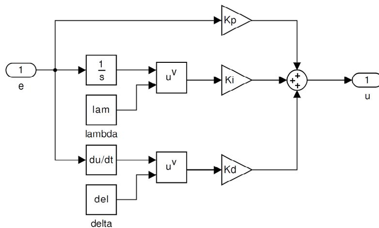
Figure 5: Simulink Model for FOPID
