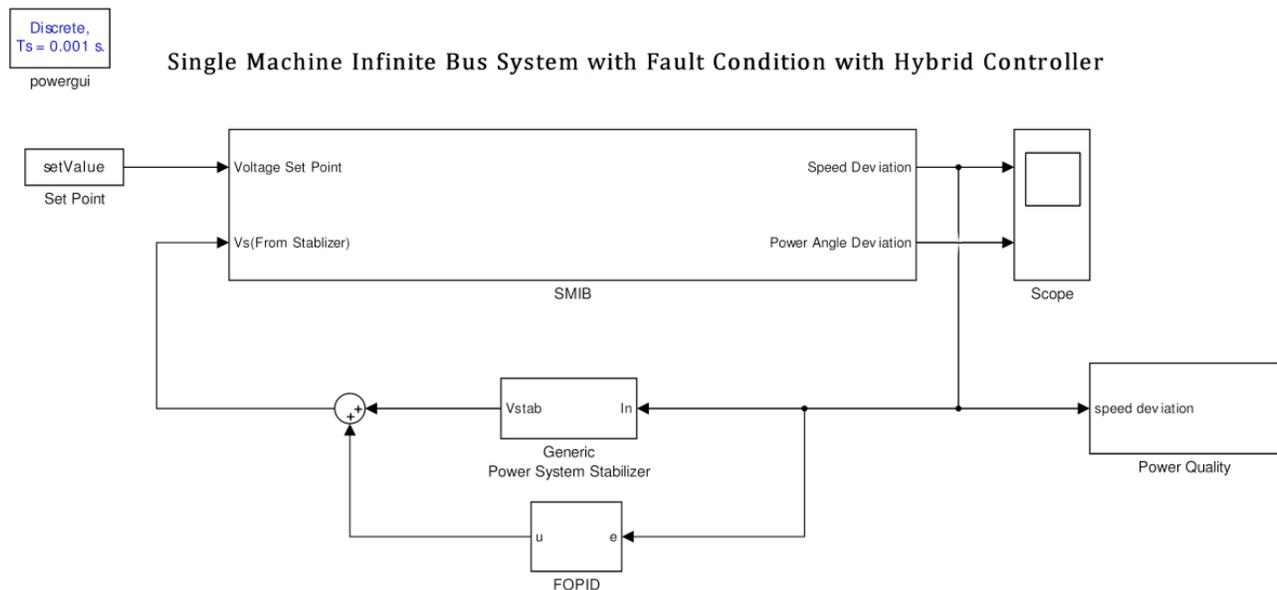
Figure 12: Simulink Model for Hybrid Approach
