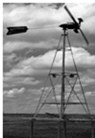
Figure 6: Wind Charger (100 W, DC, with flap air brakes). Location: USDA-ARS wind test station, Bushland, Texas
