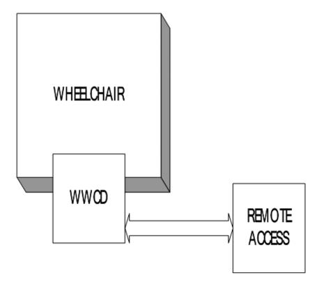
Our idea is to create wheelchair which consists of WWCD which is control by Bluetooth communication. The WWCD consists of a microcontroller camera, ultrasonic sensor and motor. Much clear flow diagram is given below.
