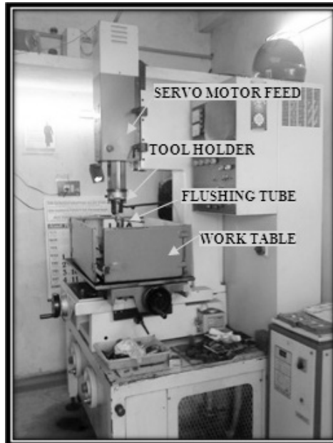
Figure 1: Die-sinking EDM arrangement
