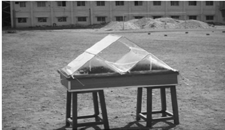
Figure 1: Photograph of double slope Tribasin solar still
