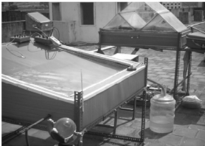
Figure 2: Photograph of experimental testing in sunny days double slope Tribasin solar still
