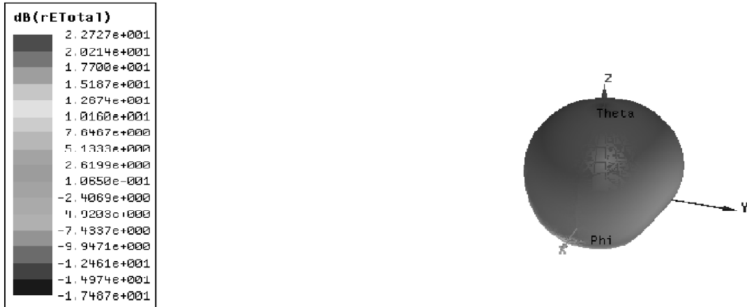
Figure 22: The rectangular patch antenna's Electric field pattern
