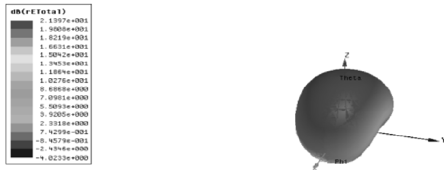
Figure 7: The rectangular patch antenna's electric field pattern
