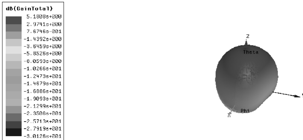
Figure 18: The rectangular patch antenna's gain
