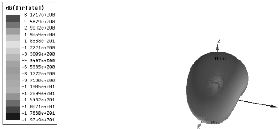
Figure 9: The rectangular patch antenna's directivity
