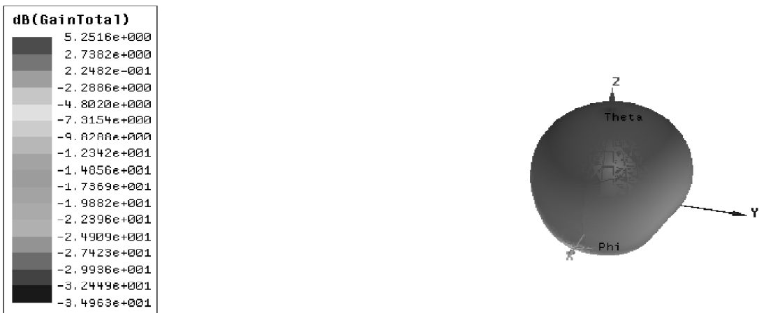
Figure 23: The rectangular patch antenna's gain
