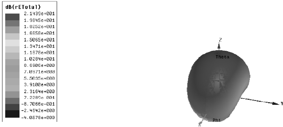
Figure 12: The rectangular patch antenna's electric field pattern
