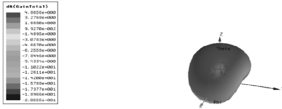
Figure 8: The rectangular patch antenna's gain
