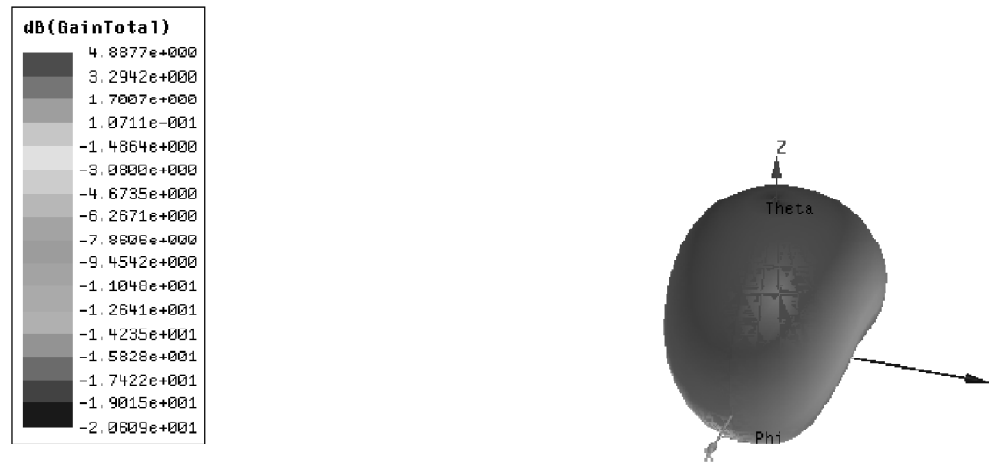
Figure 13: The rectangular patch antenna's gain
