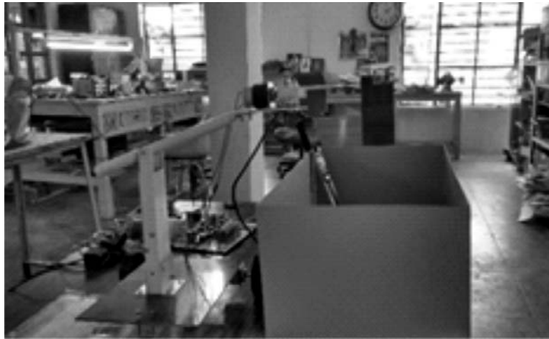
Figure 6: Hard ware model of sub assembly bay with robotic arm
