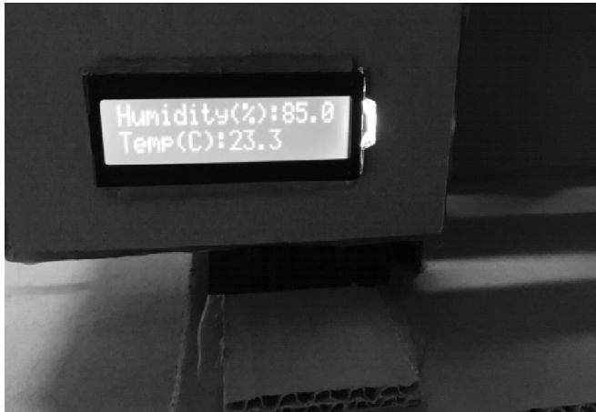
(a) The LCD panel display of the temperature sensor
