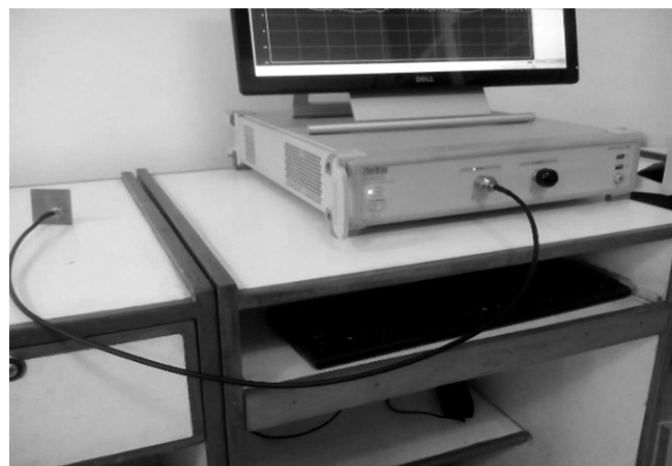
Figure 5: antenna under testing using network analyzer
