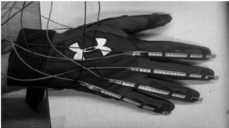
Figure 13: Gesture Glove Connections
