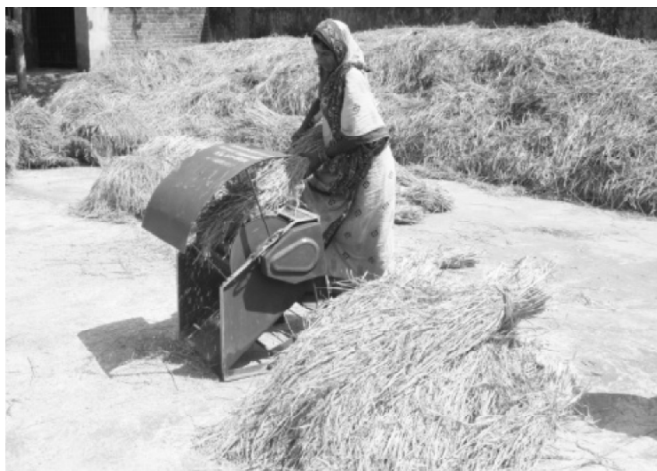
Figure 5: Pedal Thresher with Safety Cover
