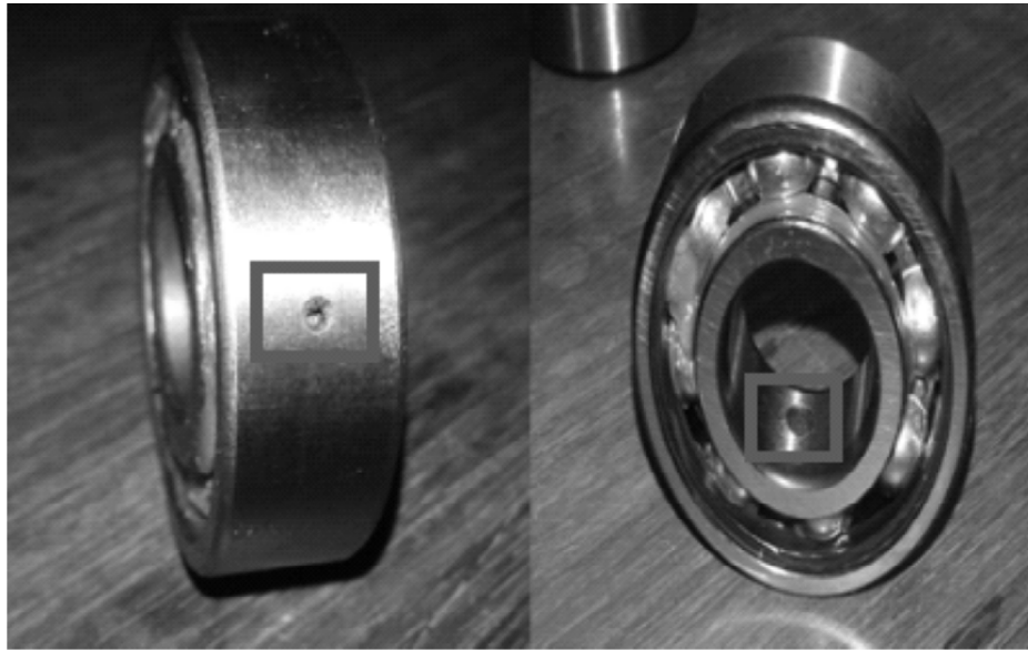
Figure 2: Ball bearings with inner race and outer race defects
