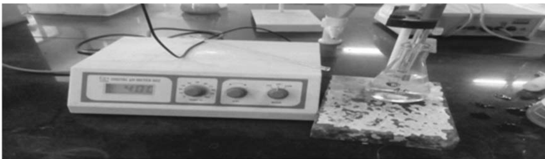
Fig. 5. Calibrating the meter to get pH of buffer solution with pH 4.00
