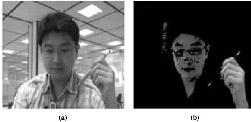
Figure 2: Instance of skin color extraction outcome (a) Original frame (b) Extracted skin color pixels
