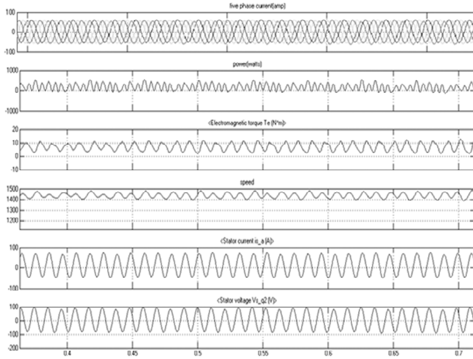
Figure 12: Performance of the PMBLDCM drive under speed 1500 rpm
