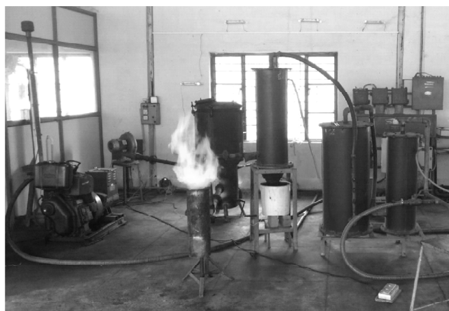
Figure 2: Downdraft gasifier - diesel engine set up in operating condition
