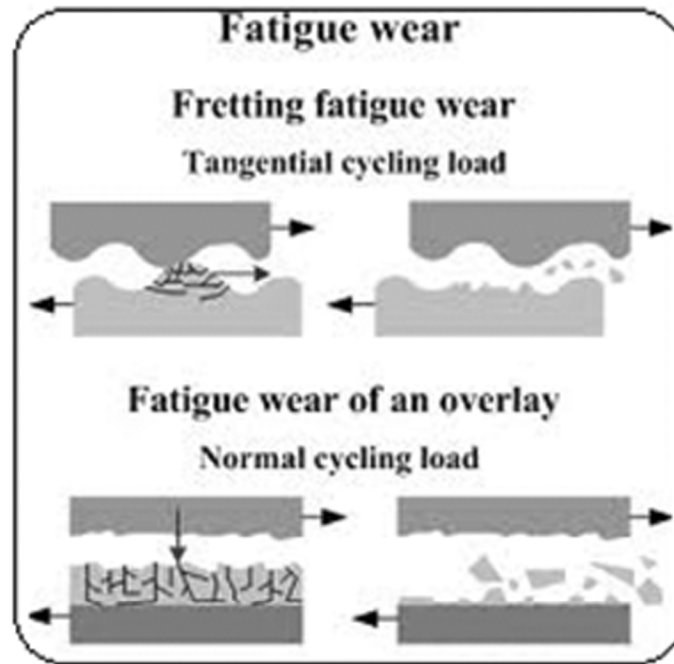
Figure 4: Fatigue Wear by Tangential and Normal Cycling Load
