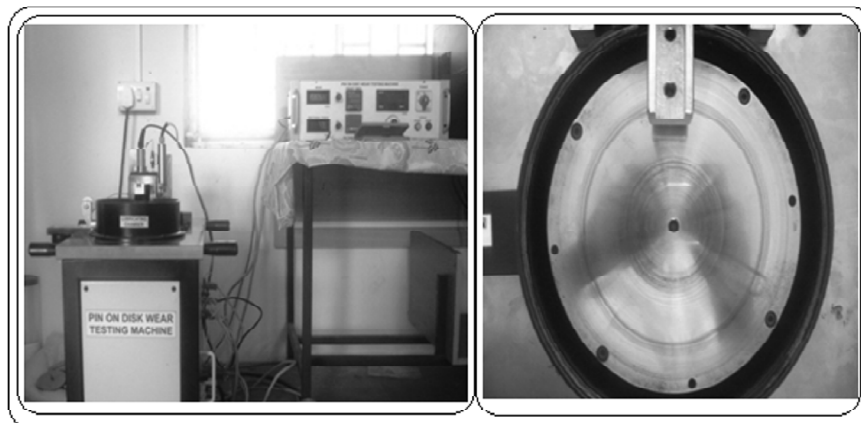
Figure 5: Pin-on-disc type Friction and Wear monitor (DUCOM; TL-20) with data acquisition system
