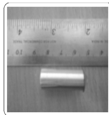
Figure 7: Casting (Job Material) for Wear Testing
