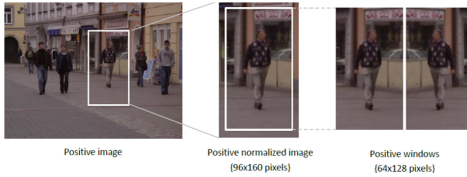
Figure 5: Generation of positive samples
