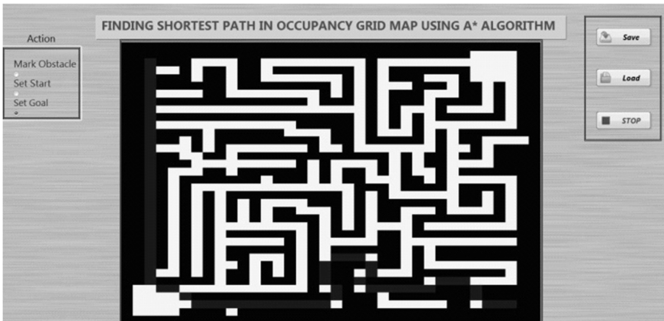
Figure 4: LabVIEW simulation for the Occupancy Grid Algorithm using A* algorithm
