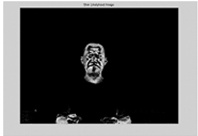
Figure 1: (b) Image segmentation into skin and non-skin regions based on Likelihood model Likelihood model
