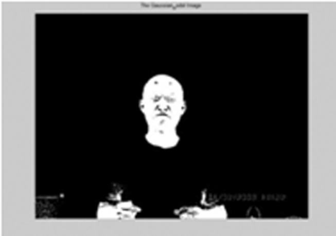
Figure 1: (a) Image segmentation into skin and non-skin regions based on Gaussian model.
