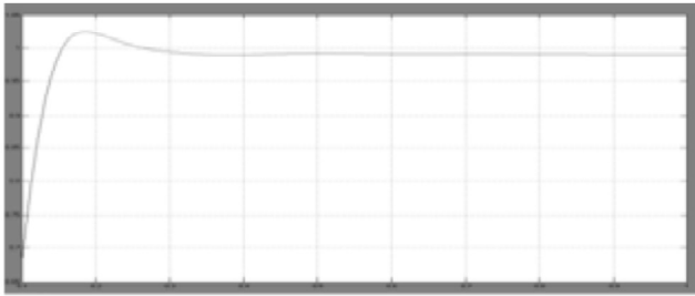
Figure 6: Performance parameters of the UPF rectifier using HCC at a rated wind speed of 12 m/s. (a) Input power factor of the front-end rectifier employing HCC at a rated wind speed of 12 m/s.
