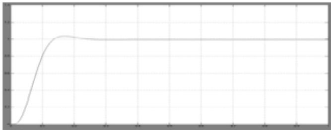
Fig. 10. Performance parameters of the UPF rectifier using HCC at a wind speed of 14 m/s. (a) Input power factor of the front-end rectifier employing HCC at a higher wind speed of 14 m/s.
