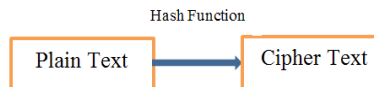
(c) Hash function (one-way cryptography). Hash functions have no key since the plaintext is not recoverable from the cipher text
