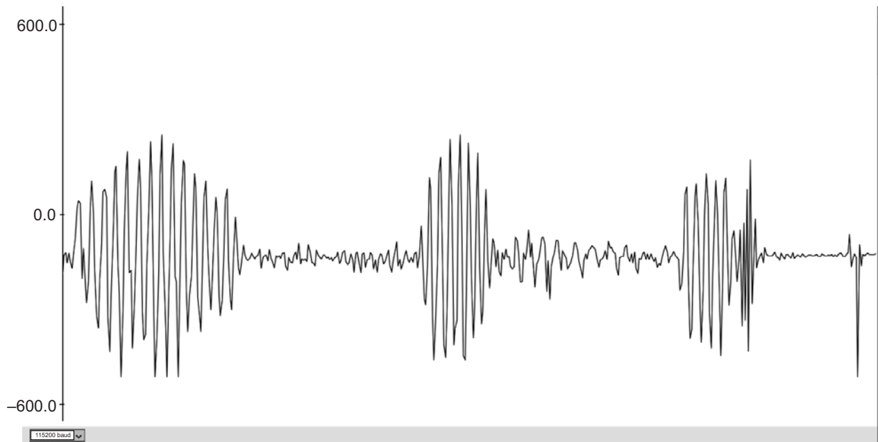
Figure 6: Vertical axis with simulated P and S waves
