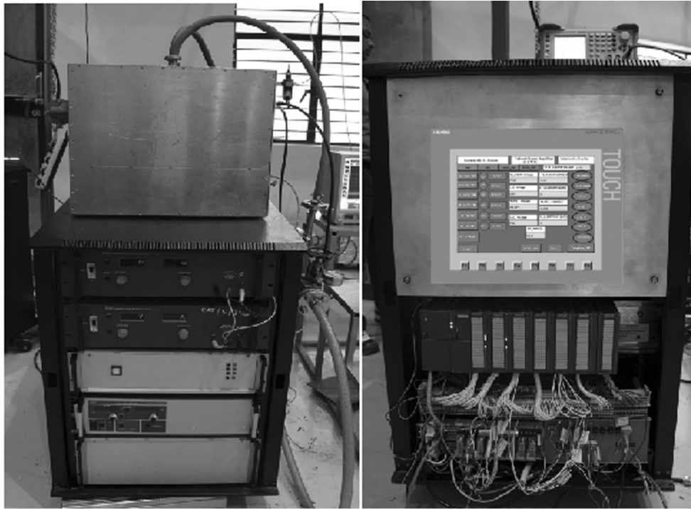
Figure 3: Tetrode tube TH561 based radio frequency (RF) high power pulse amplifier system at 1 MHz setup
