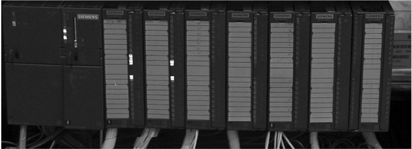
Figure 7: Employed PLC system in amplifier system.
