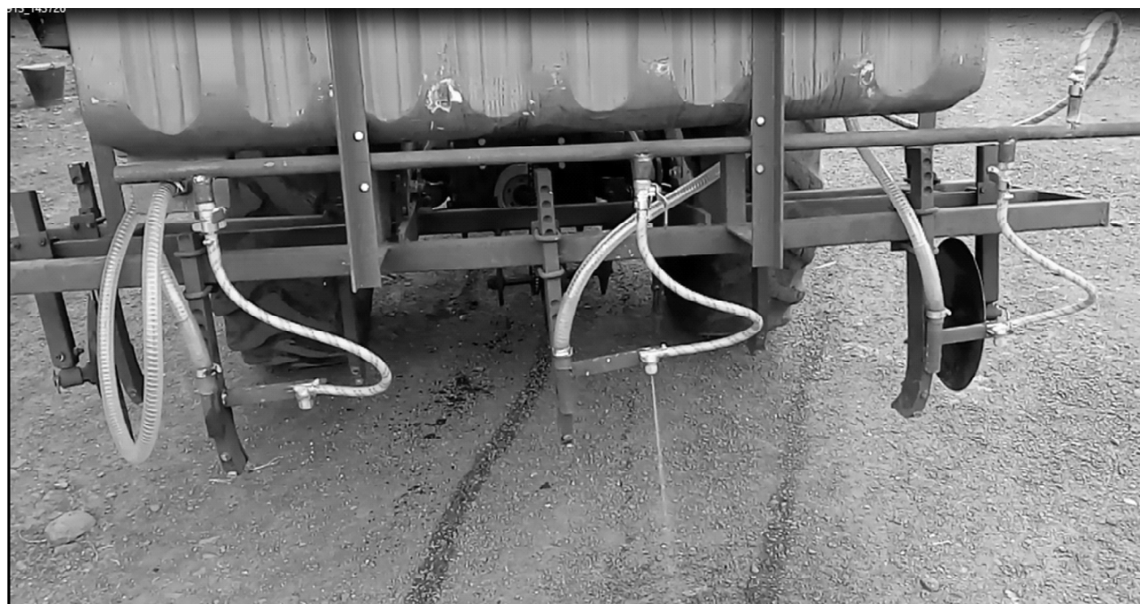
Plate: Liquid fertilizer application system on planting mechanism
