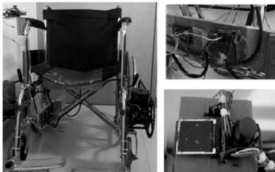
Figure 9: Mind controlled wheelchair with FRDM microcontroller and menu based embedded GUI
