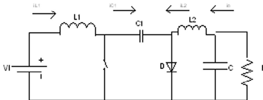
Figure 1: Non-isolated LCLC dc-dc converter
