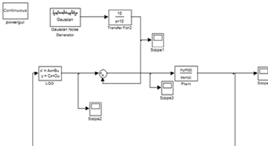
Figure 8: Simulink model of the plant with LQG regulator and low pass filter
