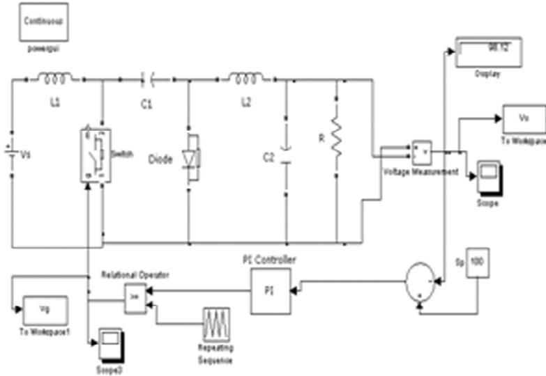
Figure 4: Simulink model of converter with controller
