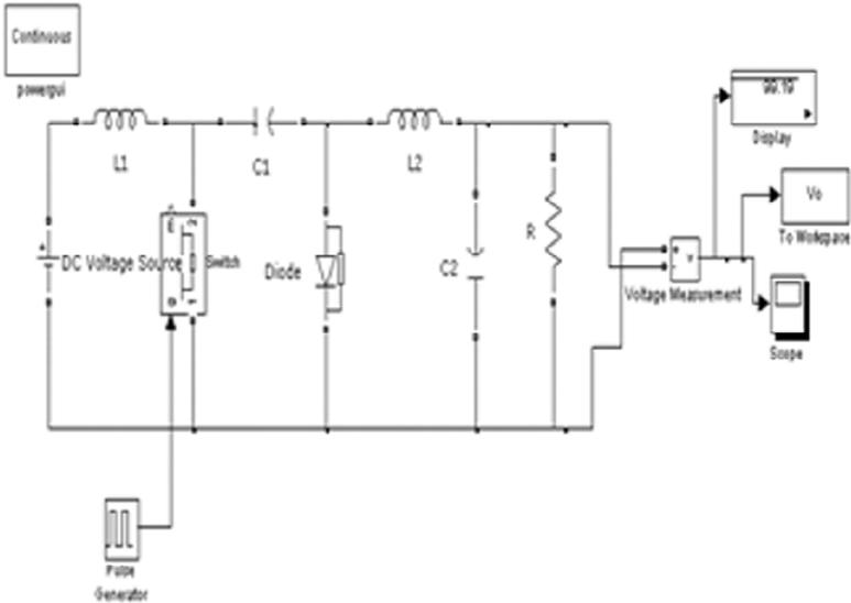
Figure 2: Open loop model of non isolated LCLC converter
