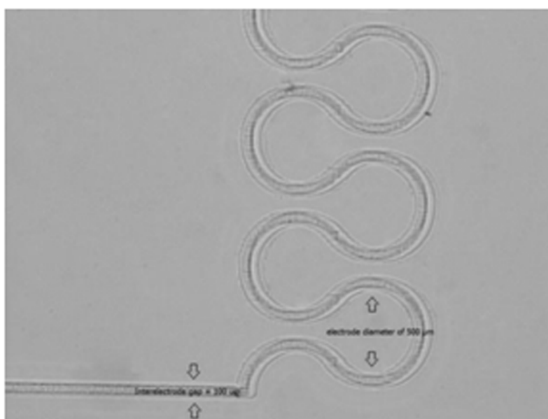
Figure 2: Zipper electrode with 500 \mu\text{m} diameter, 100 \mu\text{m} interelectrode gap fabricated using laser technology
