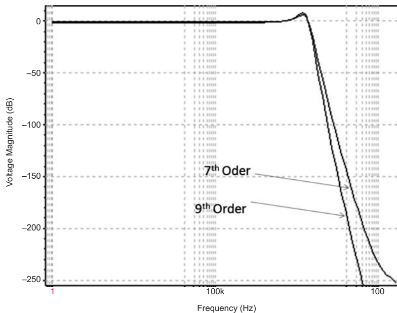
Figure 15: Response of low pass filter as a function of filter order
