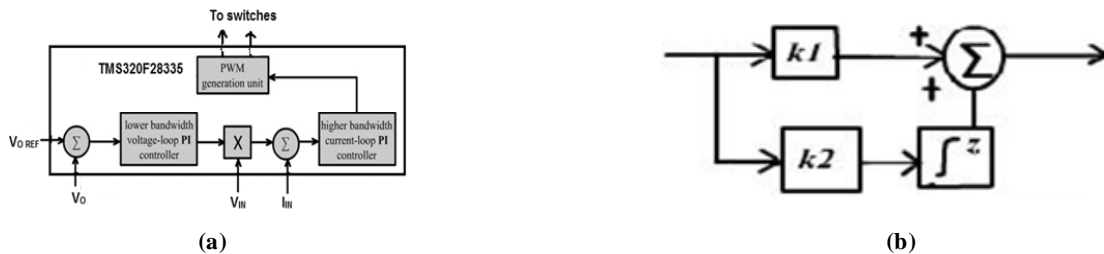
Figure 2: (a) Digital PI control implementation of AC/DC converter. (b) PI controller in z-domain using bilinear transformation
