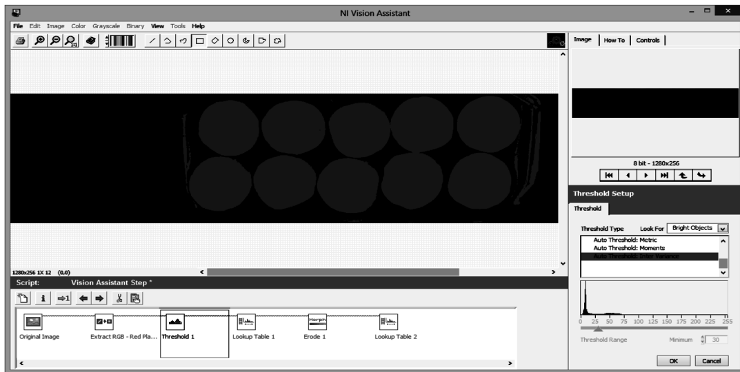
Figure 5: Binary image showing foreground and background using Otsu’s algorithm
