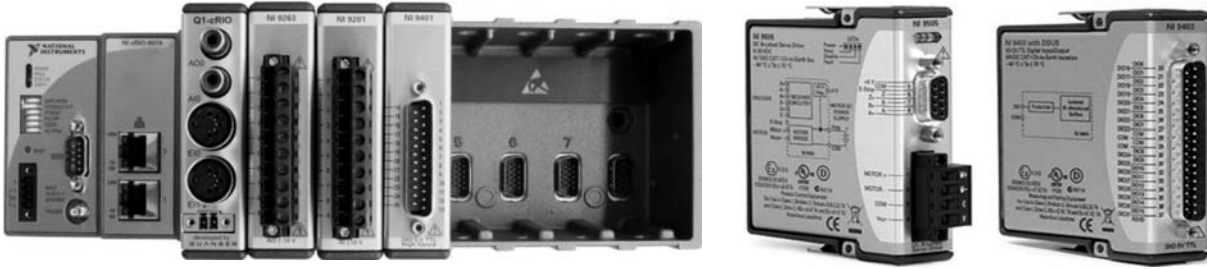
Figure 3: Illustrative Photographs of cRIO Controllers and C-series Modules
