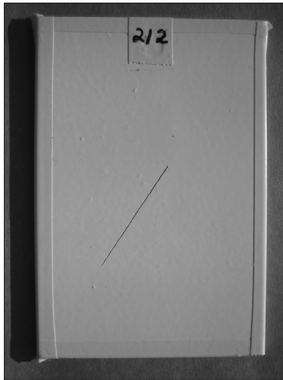
Figure 1: A Coated Test Panel with a Diagonal Scribe
