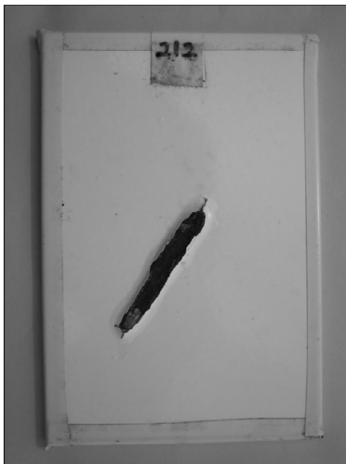
Figure 3: Rust Creepage Developed at Scribe After the Test
