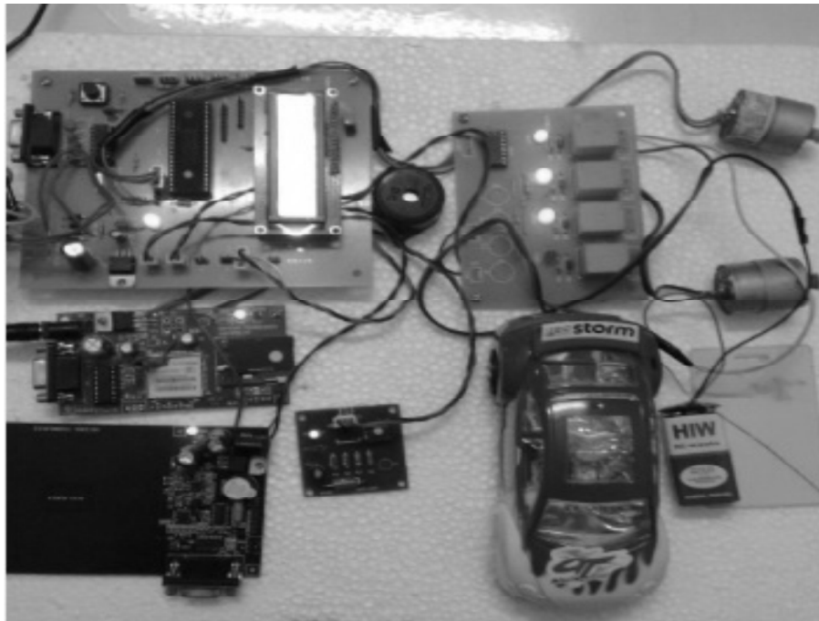
Figure 6: Vibration sensor –microcontroller interface circuit
