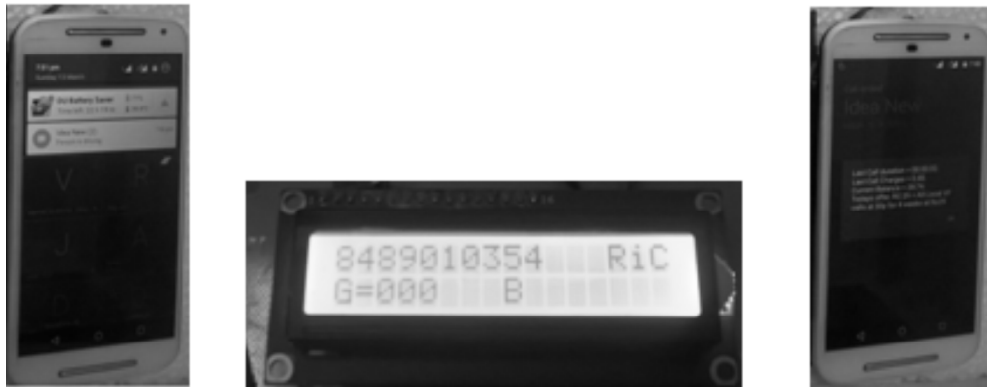
Figure 8: Phone call and message indication setup
