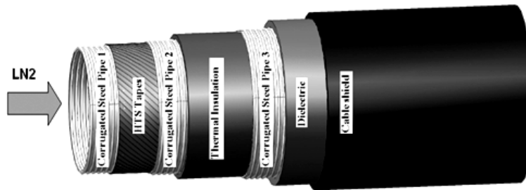
Figure 1: Warm dielectric Coaxial cable
