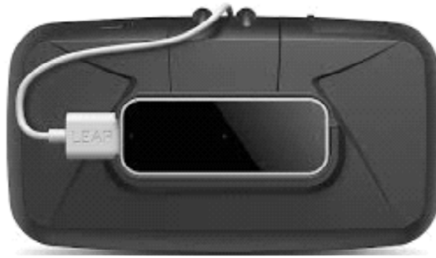
Figure 2: Leap Motion Sensor
