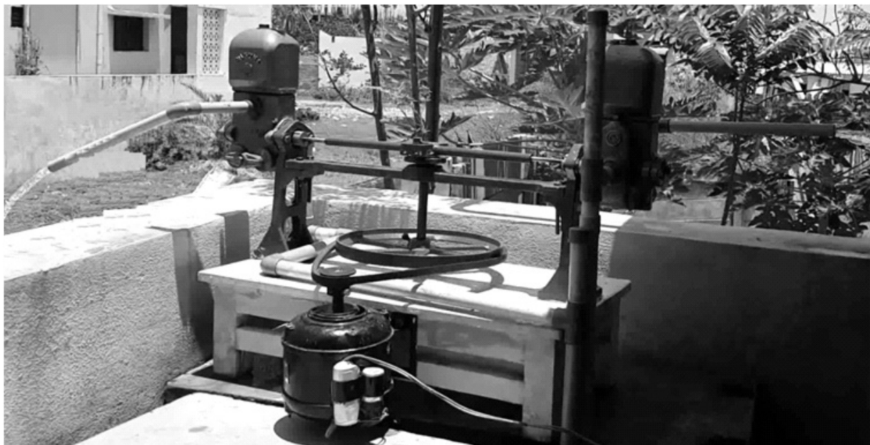
Figure 3: Fabricated Duplex Reciprocating Pump
