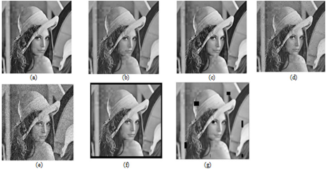
Figure 6: Watermarked images after attacks (a) Resize (50%) (b) JPEG compression (Q = 40) (c) LPF (window 3x3) (d) s & p ( 0.01) (e) Gaussian noise (0.01) (f) Cropping (10%) (g) Tampering
