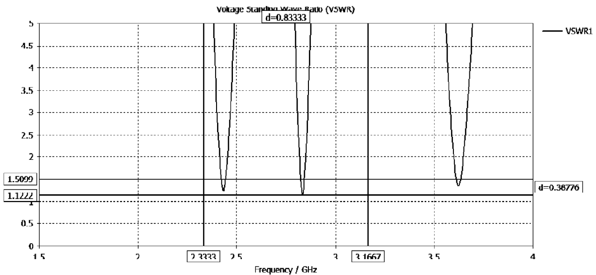
Figure 11: VSWR of the proposed patch
