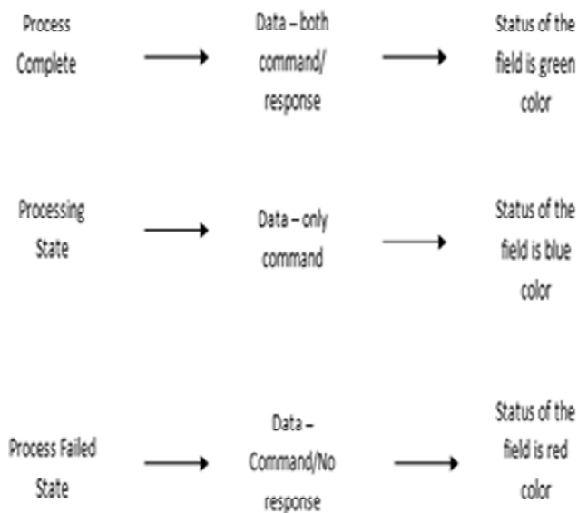
Figure 7: Flowchart representing the status of ESP fields.
