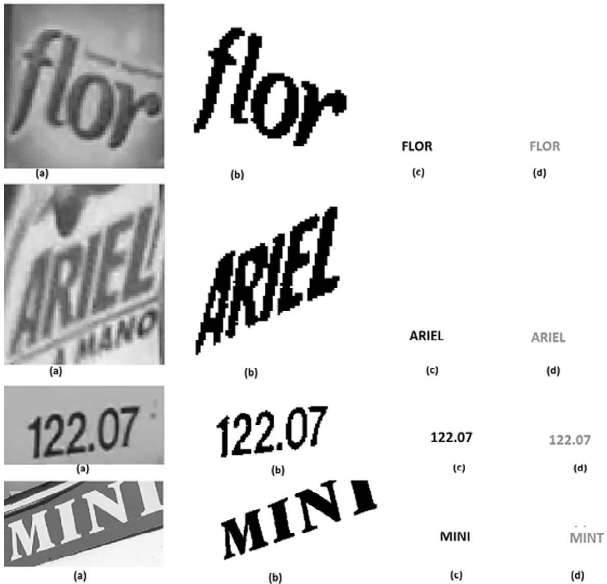
Figure 7: Text extraction steps. (a) Shows cropped text area from the video frame, (b) binary image of text area after background subtraction and histogram matching. (c) Extracted text from the binary text blocks, (d) text correction using minimum distance matching from available dictionary.
