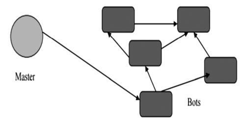
'neighbours', and any command received by a bot from one in every of its neighbours are going to be sent on to the others, distributing it across the zombie network. During this case, a hacker must have access to a minimum of one pc on the zombie network to be able to control the complete botnet.
