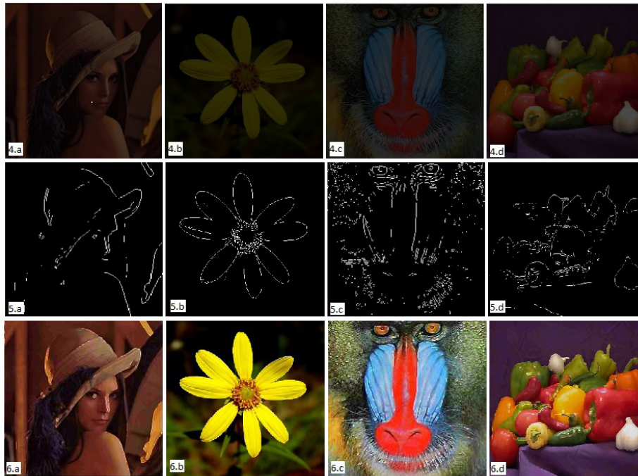
Figure 4a-4d: Low contrast images. Figure 5a-5d: extracted features. Figure 6a-6d: DSR enhanced and foreground sharpened images.
