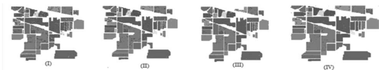
Fig. 4. Classification map for 10 % (I) without processing (Overall accuracy- 71.72 %), (II) denoising using T.V algorithm (Overall accuracy- 78.27 %), (III) denoising using wavelets (Overall accuracy- 81.12 %), (IV) denoising using \lambda_1 norm (Overall accuracy- 82.63 %),
