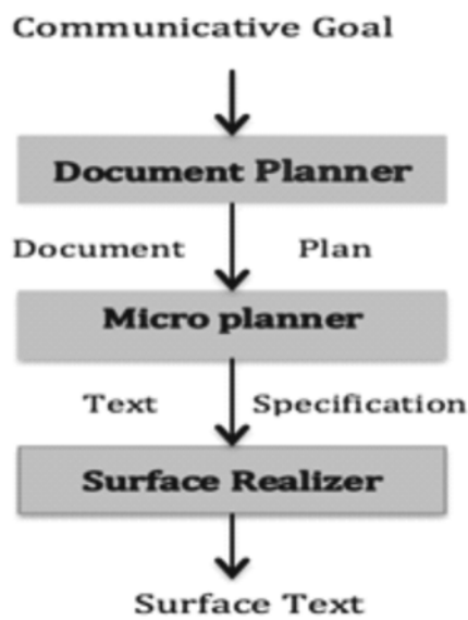
Fig. 1a – Pipeline Architecture ,
